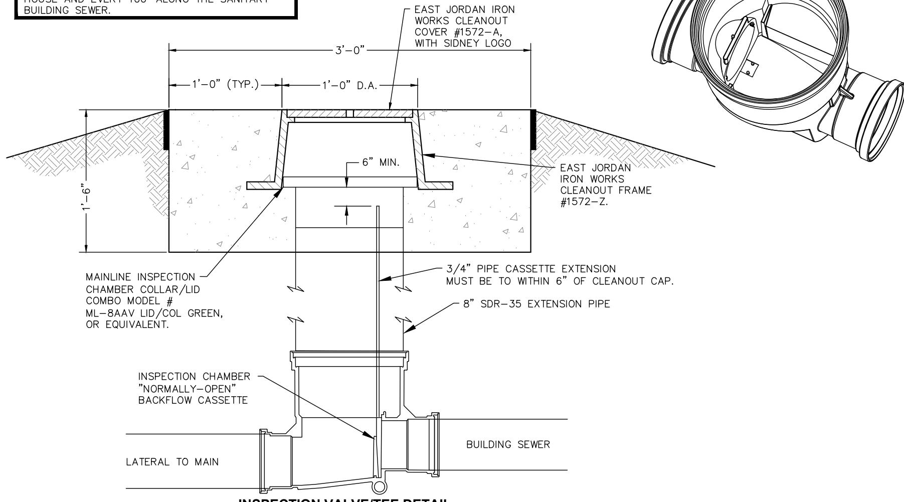
INSPECTION VALVE/TEE SHALL BE MANUFACTURED BY MAINLINE OR AN APPROVED EQUIVALENT. INSPECTION VALVE/TEE PLACED IN RIGHT-OF-WAY INLINE WITH WATER METER PREFERRED.
