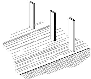
B. EXCAVATE A 4" x 4" TRENCH UP SLOPE ALONG THE LINE OF STAKES.
