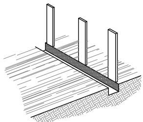
C. STAPLE FILTER MATERIAL ON UP SLOPE SIDE OF STAKES AND EXTEND IT INTO THE TRENCH. WHEN JOINTS ARE NECESSARY, OVERLAP MATERIAL BETWEEN 2 STAKES AND FASTEN SECURELY.
