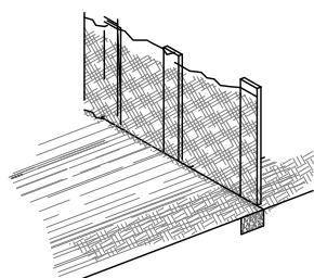
D. BACKFILL AND COMPACT THE EXCAVATED SOIL.
